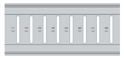
Mounting hole 1 For Panel width: 1018-1052mm Mounting hole 2 For Panel width: 1052-1086mm Mounting hole 3 For Panel width: 1086-1120mm Mounting hole 4 For Panel width: 1120-1155mm Mounting hole 5 For Panel width: 1155-1190mm
